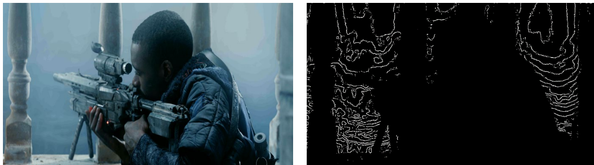
Figure 2 - Video frame (left) with banding artifacts, and banding map (right) created by an objective banding detection algorithm.
