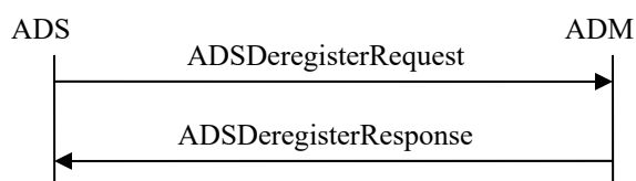
Figure 40: ADS Initiated Deregistration Message Exchange
