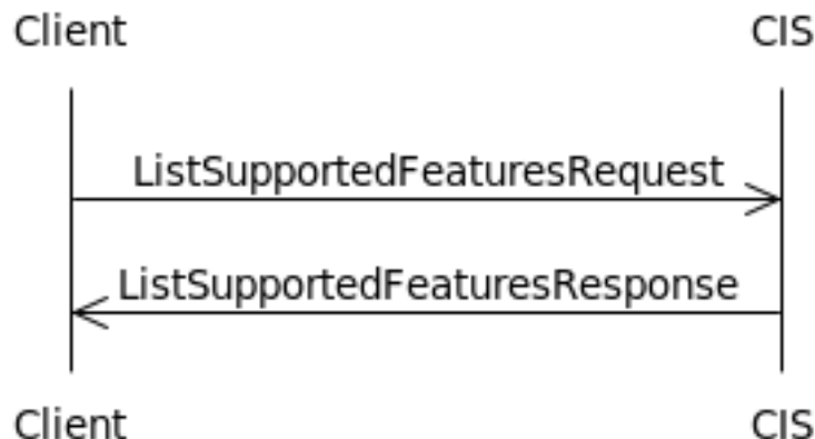
Figure 71: CIS Discovery Sequence Diagram
