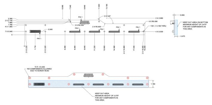
Figure 15 – High-Speed Lid Backplane Dimensions
