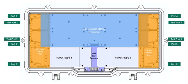
Figure 2 – GAP Base with a Full-Size Base Module (Tray Style)
