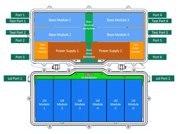
Figure 1 – GAP Reference Architecture
