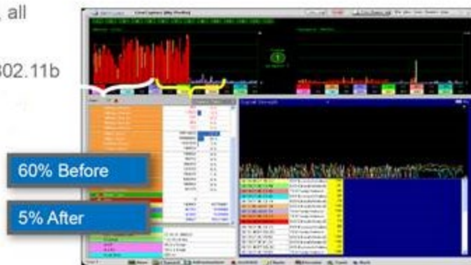
Figure 8 - SSIDs and Low Rates Consume Air Time
